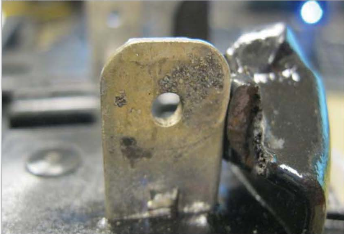
Figure 1. Pitting and Discoloration of a Hot Socket Meter Stab Returned from the Field
