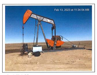
Gaskill 1-35 API# 15-181-20618-00-00 GPS: 39.39819, -101.42572 962' NSL & 4670' WEL SE NW SW SW 35-7-37W (Active, up stroke)
