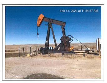
Quenzer 2-27 API# 15-181-20632-00-00 GPS: 39.41865, -101.43150 3178' NSL & 1047' WEL NW SW SE NE 27-7-37W (Active, up stroke)
