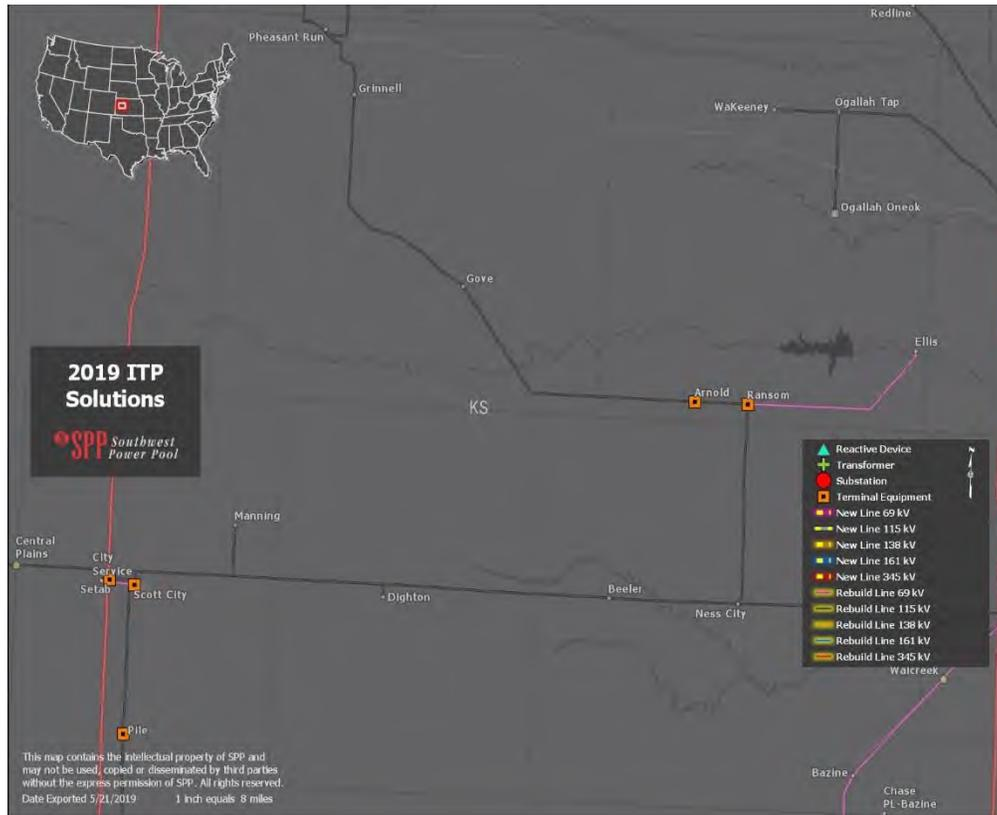
Figure 7.26: Arnold-Ransom and Pile-Scott City-Setab 115 kV terminal equipment
