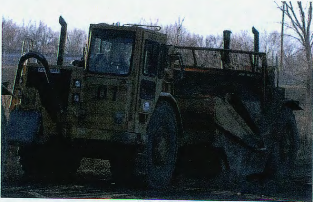
Exhibit 1-3: Paddle scraper machine that damaged pipeline.
