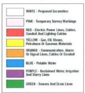
Dig With Care! The paint and flags placed by the utility company indicate the approximate location of their facilities, which may be anywhere in a 2 foot (24") tolerance zone on either side of the line of paint or flags.
