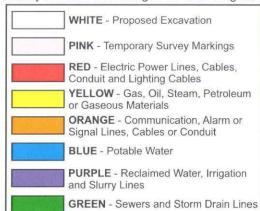
Underground facility members will use stakes, flags, paint or other suitable materials in varying combinations dependent upon the type of surface to be marked. These marks will be in sufficient quantity to clearly identify the routes of the facility. The markings may also include the initials of the underground facility owner.
