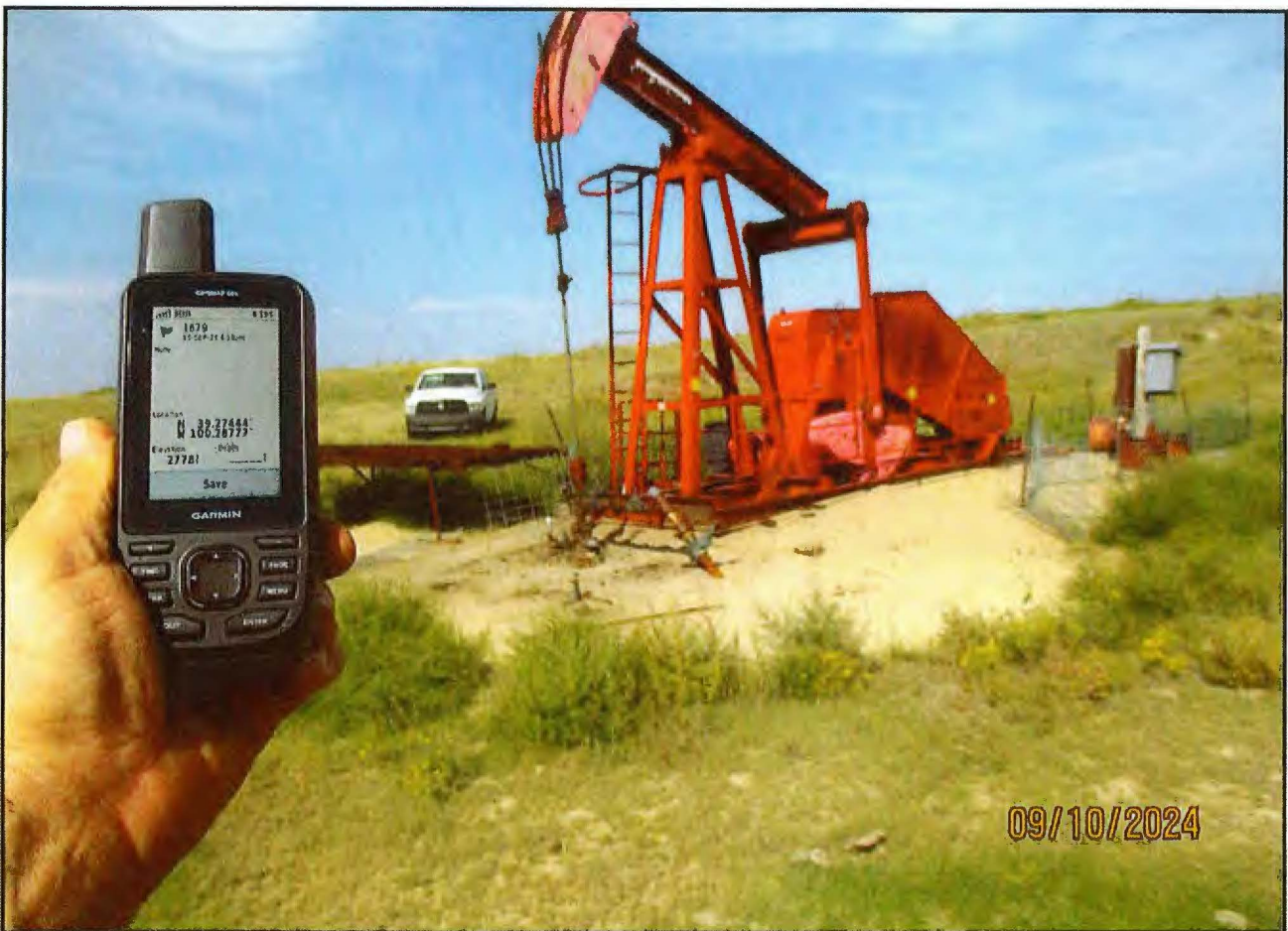
Above: View of the Breeden # 8 located SE-SW-NE-NW/4 Sec. 13-9-27W. GPS: 39.27444N & -100.28777W, 4291' FSL & 3626' FEL. The well is currently TA'd however, it may have been used to inject brine down the well. Note the lack of weight on the bridle reins. The lead line valve closest to the ground was in the closed position. The check valve allowed fluid to pass through and enter the flo-tee and fall down the tubing. The chimney valve on the wellhead was in the closed position. When the bleeder valve was open on the flo-tee it was found to be on a very strong vacuum. When the lead line valve was opened a rush of fluid could be heard passing from the lead line and into the tubing. The check valve may have been altered to allow fluid to pass through. A flapper from a 3" check valve was found inside of the pumping unit frame.
