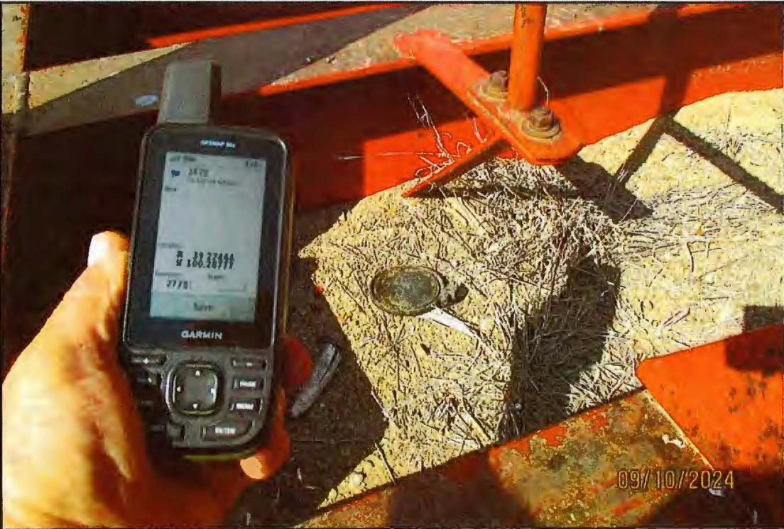
Below: View of the check valve flapper that was located inside the pumping unit frame. When opening the lead line at the wellhead, the check valve sounded as if there was a flapper installed. It is possible that the check valve may have been altered to allow fluid to pass through.
