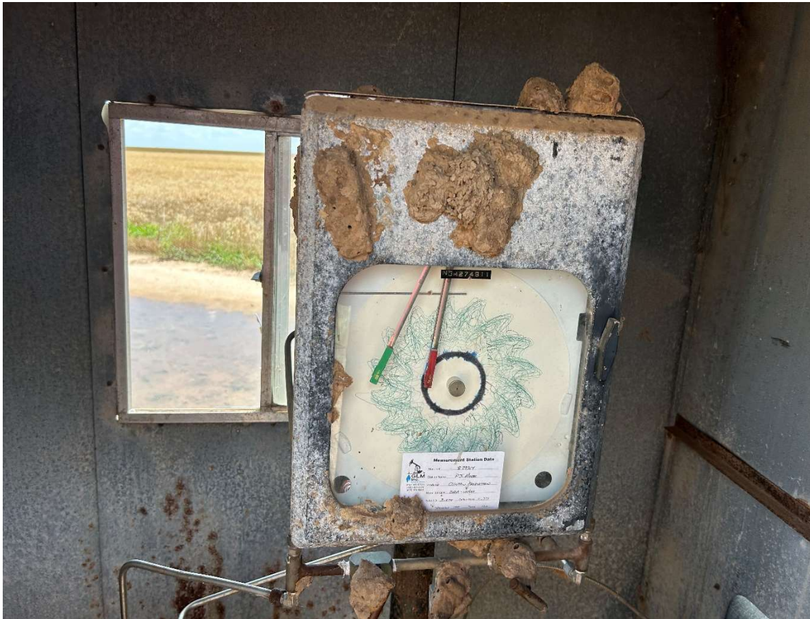
Barton meter shows no flow, chart has been left on meter with many rotations in the same position. Also chart was put on backwards to record on the blank side of chart.
