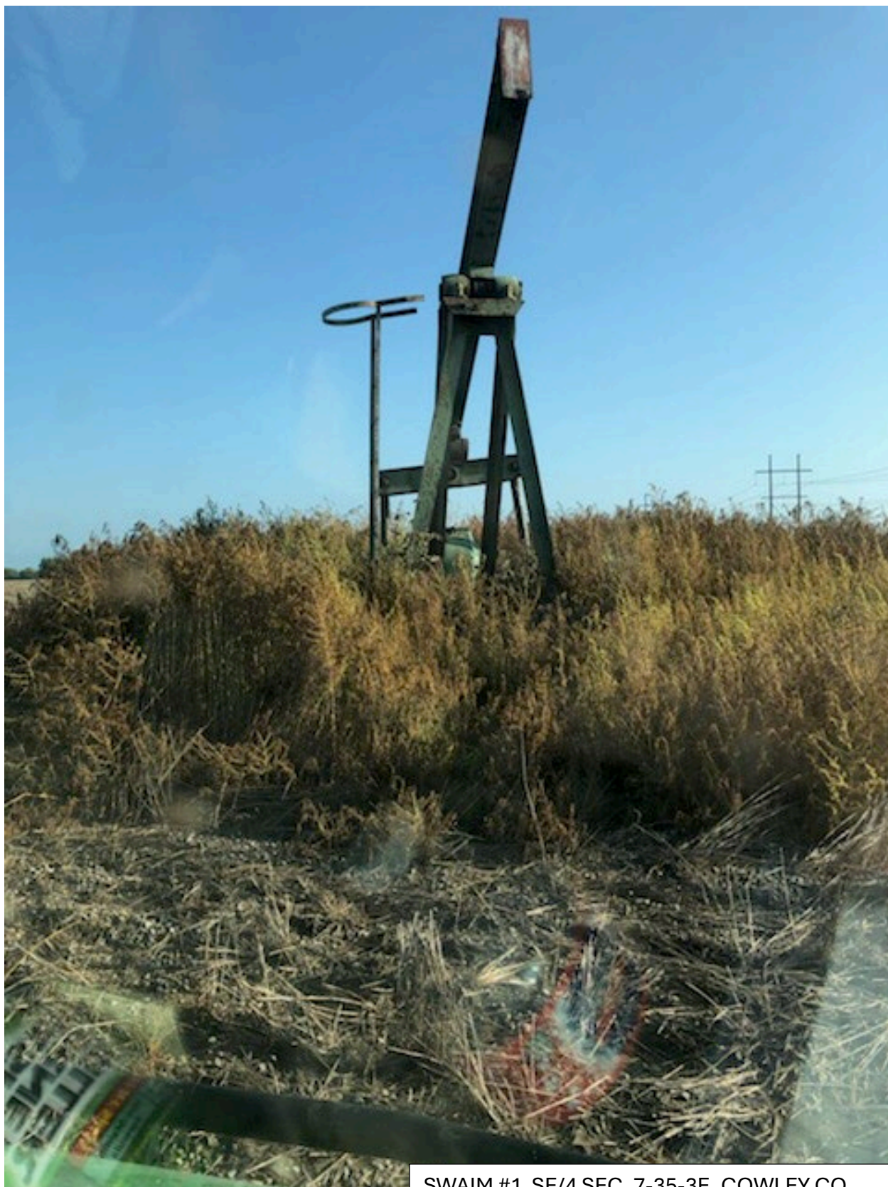
SWAIM #1 SE/4 SEC. 7-35-3E, COWLEY CO. API 15-035-23624-0000 1330' FSL 1670'FEL GAS WELL, OPEN ENDED 5.5" CASING DATE: 8-14-2020 DUANE KRUEGER
