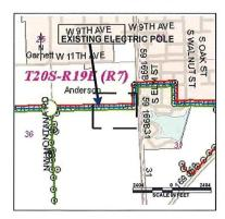
An area 250 Feet in width, being 125 Feet on each side of the following described line. Commencing at S41°31'58.227"W a distance of 170 Feet, more or less, to the POINT OF BEGINNING from EXISTING ELECTRIC POLE at approximately 38°16'11.980"N, 95°15'12.322"W, thence N88°43'6.314"E a distance of 1205 Feet, more or less, thus to the end point.
