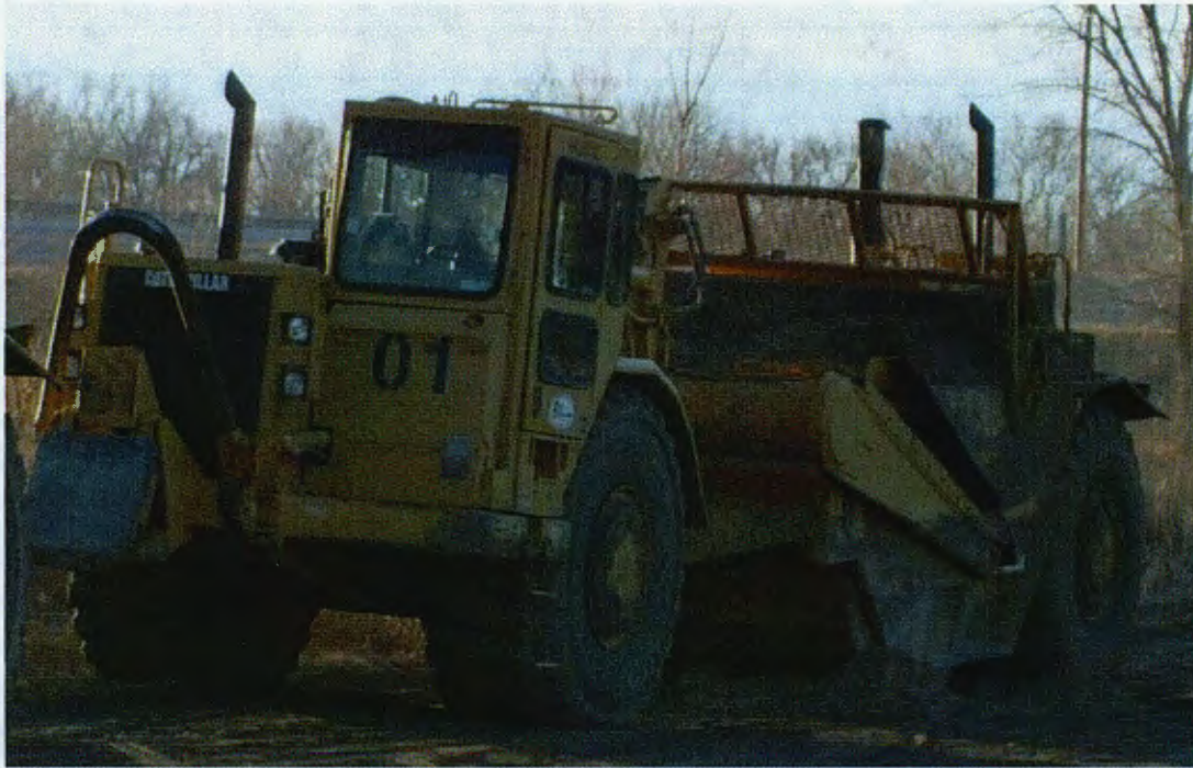
Exhibit 1-3: Paddle scraper machine that damaged pipeline.
