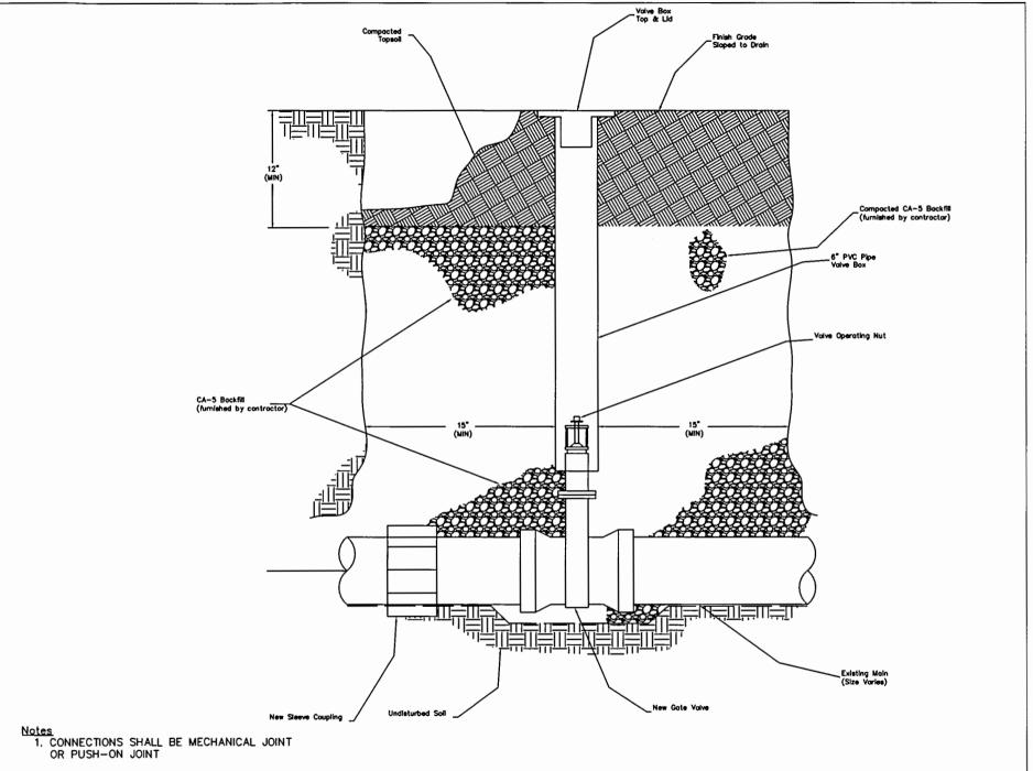
VALVE STEM EXTENSIONS SHALL BE INSTALLED ON VALVE INSTALLATIONS AS REQUIRED TO MAINTAIN A MAXIMUM OF 5' FROM FINISH GRADE TO VALVE NUT.
