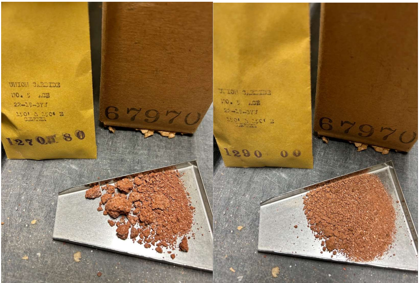
Cuttings from the AEC Test Hole #5 NE Sec. 22-T19S-R37W Wichita County, KS. The sample on the left is from a depth of 1,270' to 1,280' and the sample on the right is from a depth of 1,290' to 1,300'
