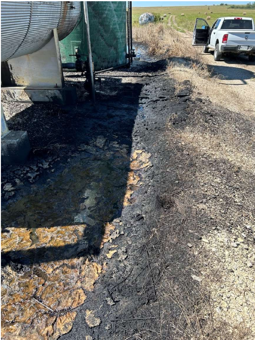
Everglow Energy, LLC KCC #35495 William O. Olsen Tank Battery SW/4 Sec. 26-15-9E, Morris Co., KS Discharge around the separating equipment. Date: September 3, 2024
