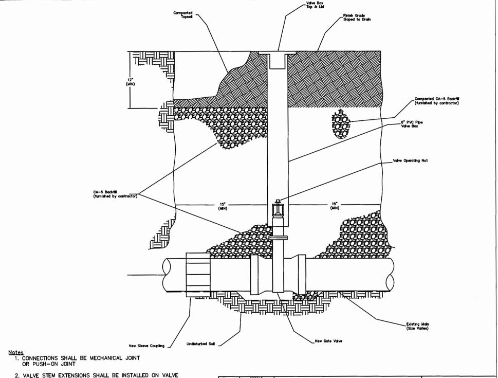
2. VALVE STEM EXTENSIONS SHALL BE INSTALLED ON VALVE INSTALLATIONS AS REQUIRED TO MAINTAIN A MAXIMUM OF 5' FROM FINISH GRADE TO VALVE NUT.
