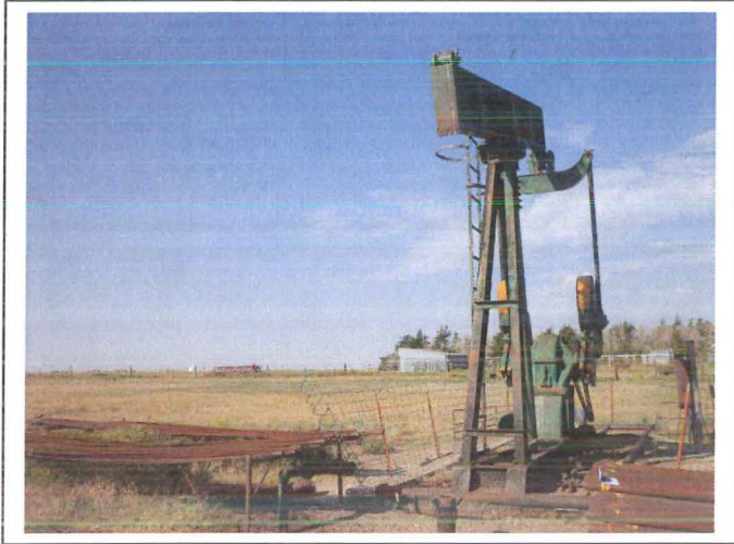
Photo taken September 13, 2017. The Schmeidler-A well # 8 located in the SW NE NW still has an open hole with rods and tubing located at the well site. API # 15-051-20626-00- 00.
