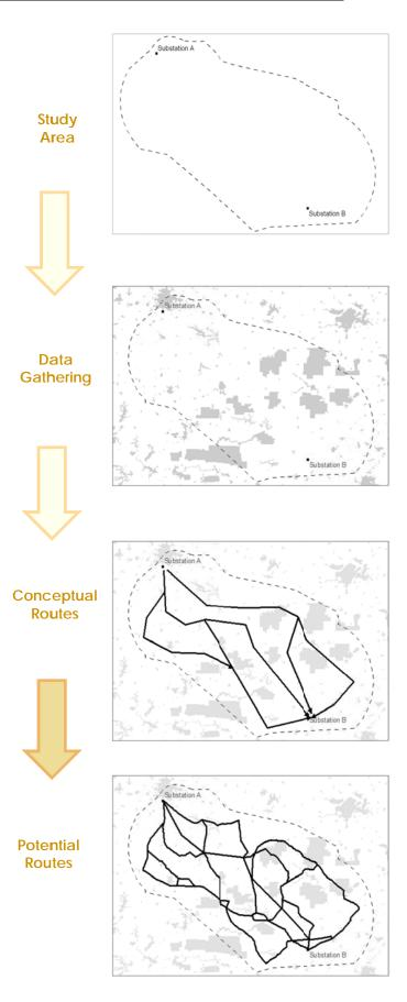
Where two or more Potential Routes intersect, a **node** is created, and between two nodes, a **link** is formed. Together, the Potential Routes and their interconnected links are referred to as the **Potential Route Network**. The links are numbered for identification, and evaluated independently and collectively for refinements.
